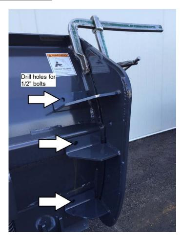
• In locations shown, drill holes for 1/2" bolts through moldboard.
