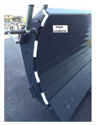
• Weld at locations shown. Weld locations are a visual guide for weld locations and minimum weld amount. Can add additional weld(s) as desired.
