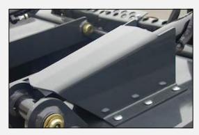
Guards protect cylinders from damage.
