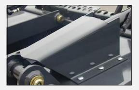
Guards protect the cylinders from damage.
