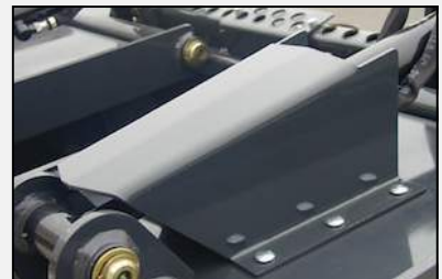
Guards protect cylinders from damage.
