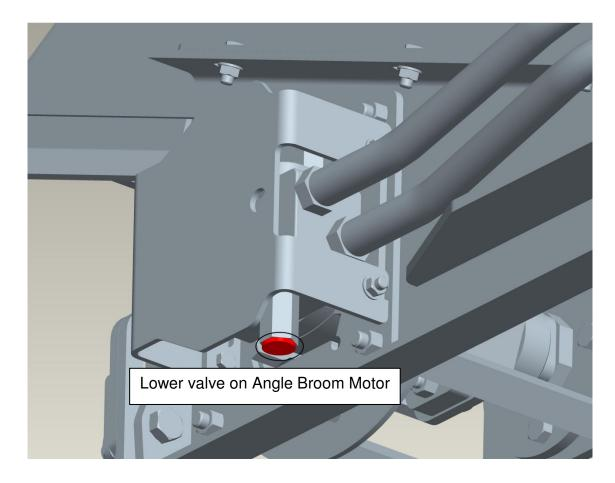
The lower valve on the angle broom can be adjusted to increase the power the broom has sweeping in the reverse direction (sweeping toward the operator).
