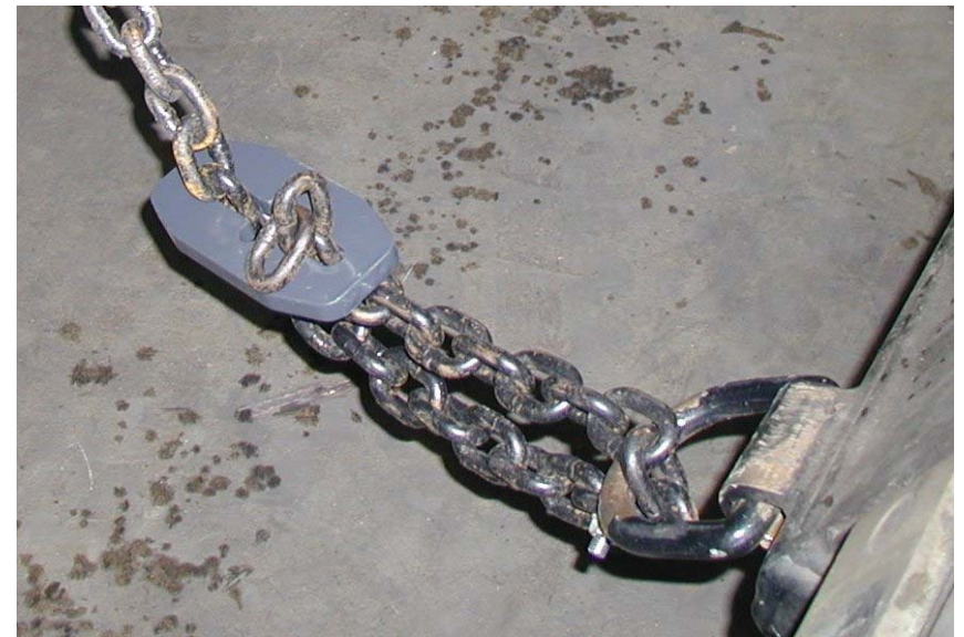
Correct installation of lift limit chain (Item #11) and lift limit retainer plate (Item #18).
