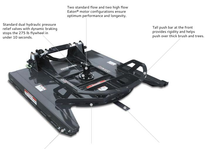
Standard replaceable front skid shoes increase the mower deck's wear life. Three-blade cutting system, mounted to a flywheel ensuring flywheel bounces off stumps rather than catching and damaging components. Double-sided, 5/8" x 5" blades can be flipped to utilize second sharpened edges.
