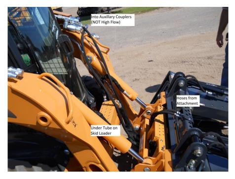
Grapple shown Center Plumb works for Case, John Deere, New Holland, Mustang, Takeuchi, and Gehl skid loaders.
