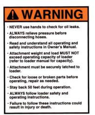
This label is located on the frame near the quick-tach. This label has several important instructions that must be followed for safe operation of this attachment.
