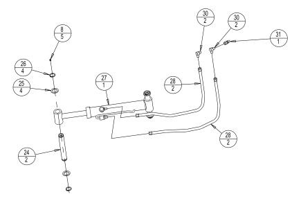
Note: Restrictor fitting (Item #31), plumbed to barrel end of cylinder.
