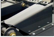
Guards protect cylinders from damage.
