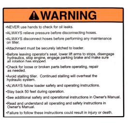
This label is located on sides of the shroud and on the frame near the quick-tach. All bystanders must stay clear during operation.
