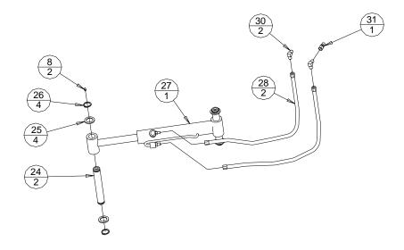
Note: Restrictor fitting (Item #31), plumbed to barrel end of cylinder.
