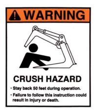
This label is located near both ends of the moldboard. Always stay clear of moldboard. Never inspect this attachment with skid loader running or with the blade raised off of the ground/pavement.
