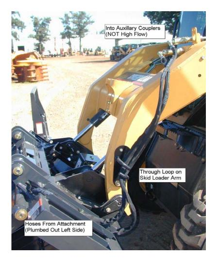
Grapple shown Left Side Plumb, works for Cat, Bobcat, Kubota, Terex and ASV.
