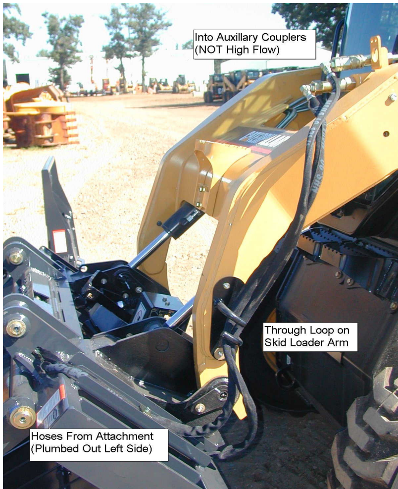
Grapple shown Left Side Plumb, works for Cat, Bobcat, Kubota, Terex and ASV.
