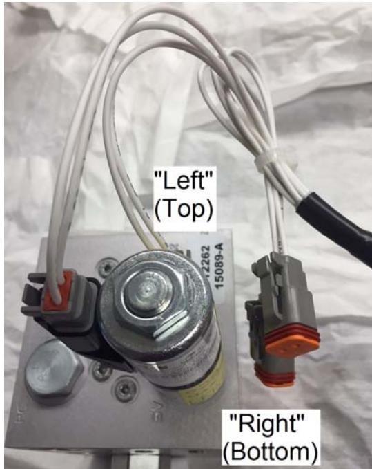
Wire Harness Installation
