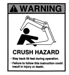
This label is located near the pivot point area on the moldboard. Always keep hands clear of dozer blade when loader hydraulic system is operational.
