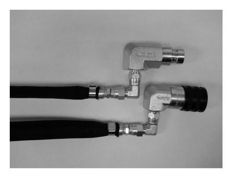
If needed, additional small elbows (Part No. 1012PP) are zip tied to the attachment and can be installed between hoses and couplers, as shown above, to improve hose routing at hydraulic coupler interface on loader. The additional elbows will not be required for most brands of skid loaders.
