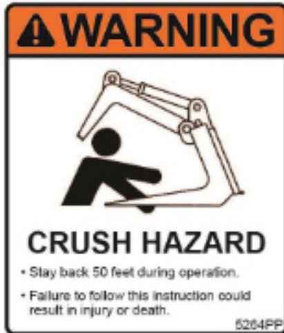
5264PP – CRUSH HAZARD WARNING LABEL
