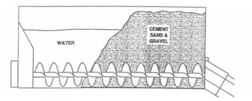
2. Run the auger in reverse. This will draw the dry material into the water and up the motor end of the bucket. The concrete mixture will roll back into the mixing material.
