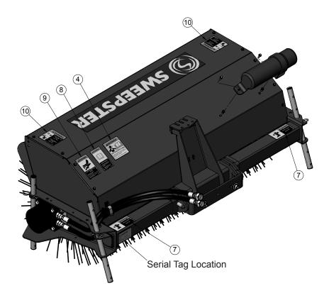
Use part numbers to order replacements for lost or damaged decals. Be sure to read all decals before operating the attachment. They contain information you need to know for both safety and longevity.
