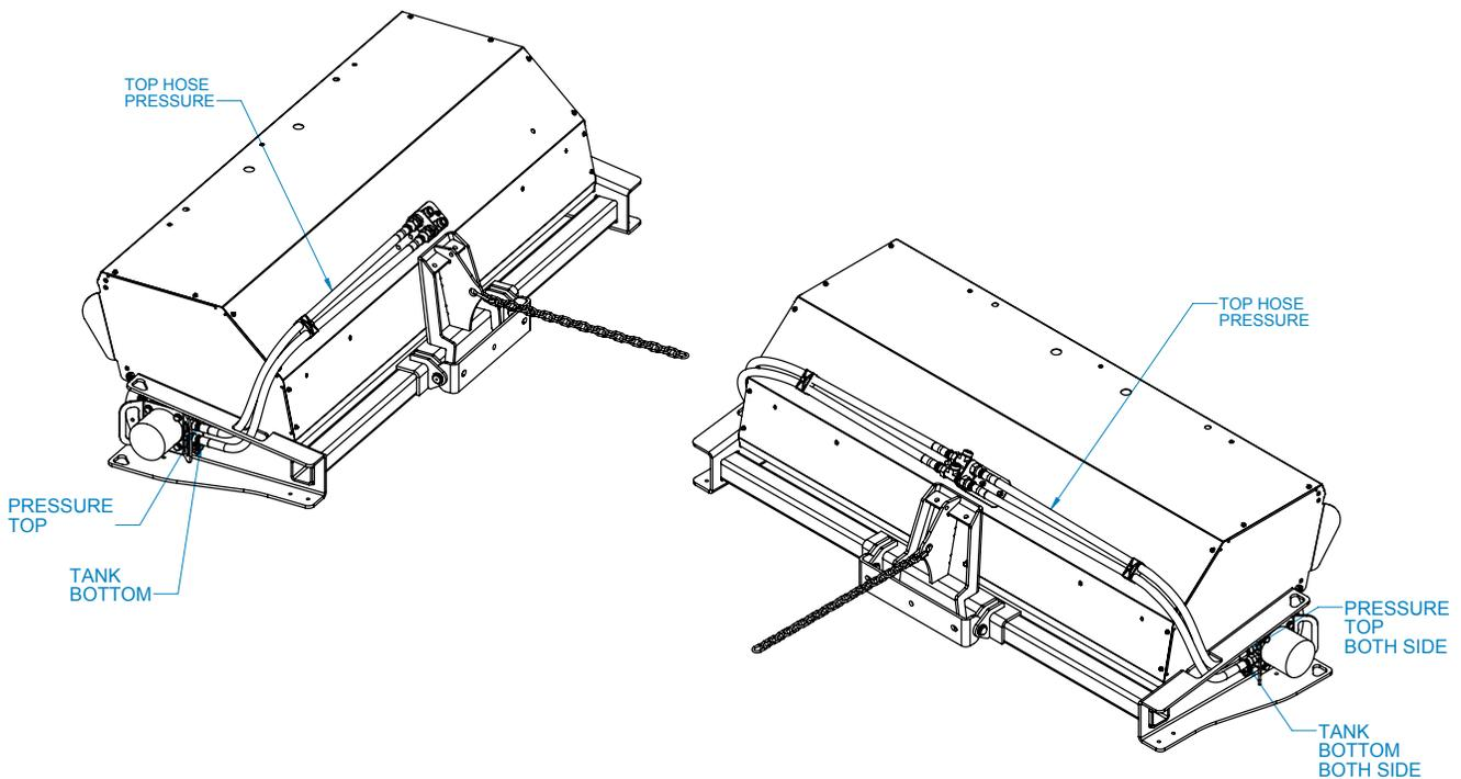
**Manual Angle:** Connect pressure line to female quick disconnect. Connect return line to male quick disconnect.
