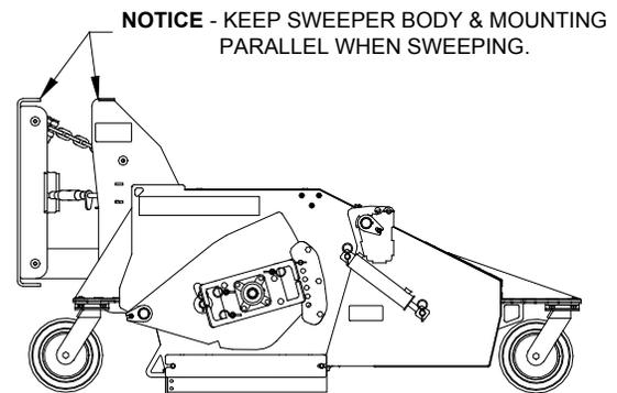
**NOTICE - AVOID SWEEPER DAMAGE.** Do not operate broom with prime mover loader arms in float. This broom is not designed to carry the weight of the prime mover loader arms.
