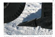
REPLACEABLE HARD SURFACED **PLOW POINT** is designed to disrupt the soil upward for easier pulling and proper silt fence installation
