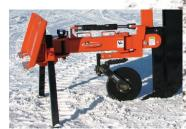
DEDICATED QUICK ATTACH SKID LOADER HITCH provides easy on and off. Both have retractable legs to keep the machines steady when unhooked.
