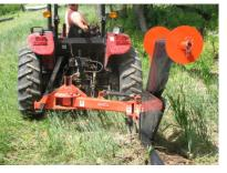
Please Note: Hyd. Top link cylinder required for proper operation of "The Silt Fence Plow' when attached to the 3 point hitch of a tractor
