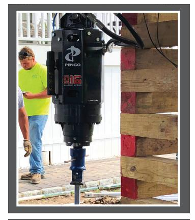
The RS-16, Pengo's newest addition to the anchor drive product line, provides significant torque capability in a compact package. The addition of a standard counterbalance valve reduces the amount of anchor kick-back often encountered during installation. The RS-16 is the perfect choice for excavators between 8T and 20T and like all Pengo anchor drives, the RS-16 is overbuilt to perform.
