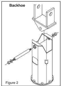
Both 1.50" diameter and 1.25" dia. pins are supplied with the drive unit. When the 1.25" diameter pin is used, insert one of the supplied bronze bushings into each of the pivot holes on the Hydraulic Drive Unit (Figure 3).
