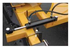
Angling capability powered by the tractor hydraulics
