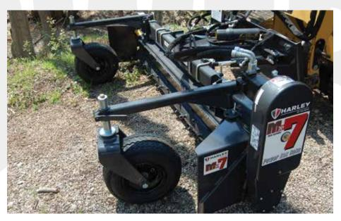
Harley comes with a standard toggle hydraulic control box. Can be ordered with an in-cab attachment controller harness.
