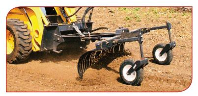
**FFC Grader Rakes,** by Paladin, have a forward facing design with a full floating hitch that allows the rake to move with the terrain. Efficiently removes debris and levels ground.
