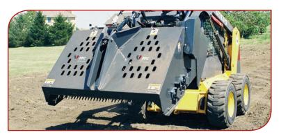
FFC AutoRake, by Paladin, an easy to use site clean-up and soil preparation attachment. This unit can be mounted on three-point configuration (tractor) and is excellent for picking up windrows in support of power box rake operations.
