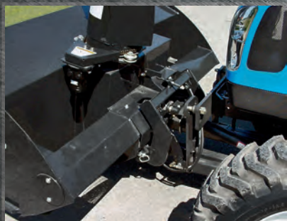
The Erskine quick attach mounting system allows for easy attachment and removal of blower unit
