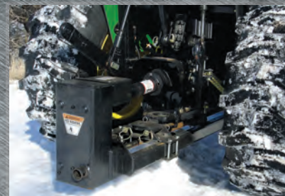
The efficient transfer case transfers power from the rear PTO to the front mounted snowblower.
