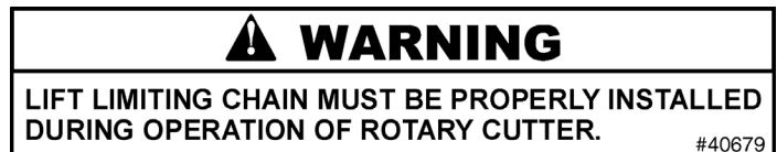
WARNING! LIFT LIMITING CHAIN PART #40679
