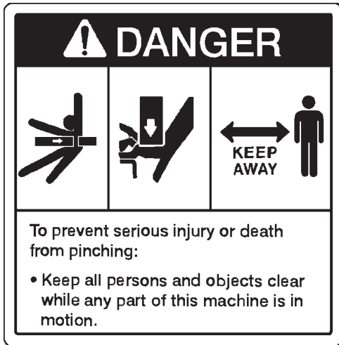
DANGER! PINCH POINT PART #40149
