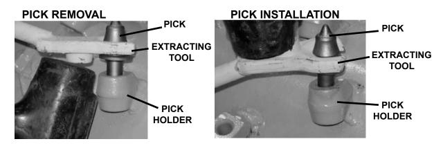
The pick is properly seated when its shoulder is against the face of the pick holder. Check to be sure the pick rotates freely.
