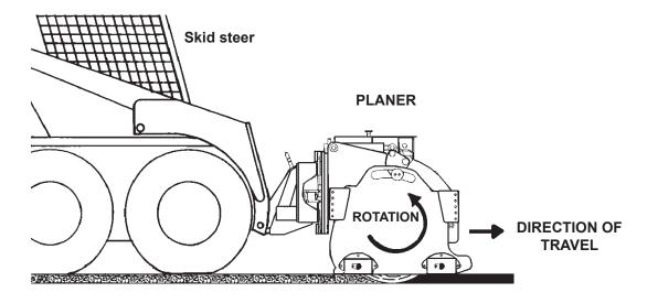
NOTE: Mill only when the skid steer is traveling forward. Do not operate when traveling in reverse.
