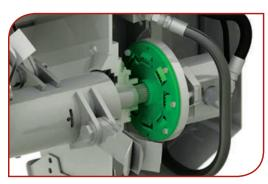
Exclusive patentpending torsion disc helps protect motor and drive assembly from damage by absorbing impact forces from the cutting blades. Bi-directional flow manifold with cross-over relief allows the operator to direct debris away from bystanders, other machinery, and buildings.
