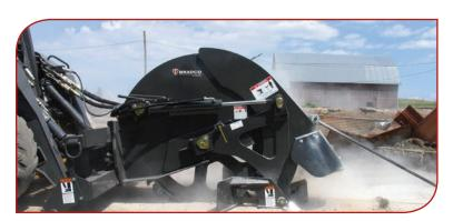
The **Bradco Rock Saw**, by Paladin, is equipped with sideshift and height adjustment features that are electrically controlled from the operator's seat.
