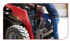
Walk-Thru carriage allows operator to step through the frame upon entry and exit.
