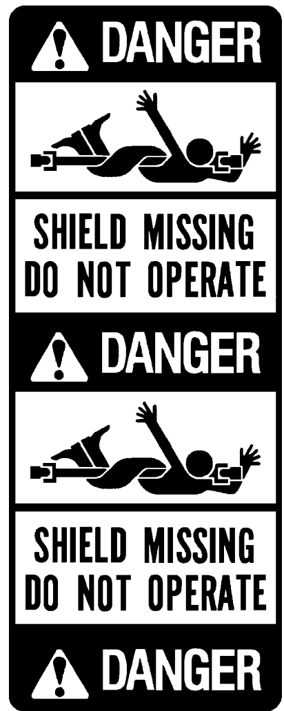
PART #4285 DANGER! SHIELD MISSING (LOCATED ON INSIDE PTO SHAFT)
